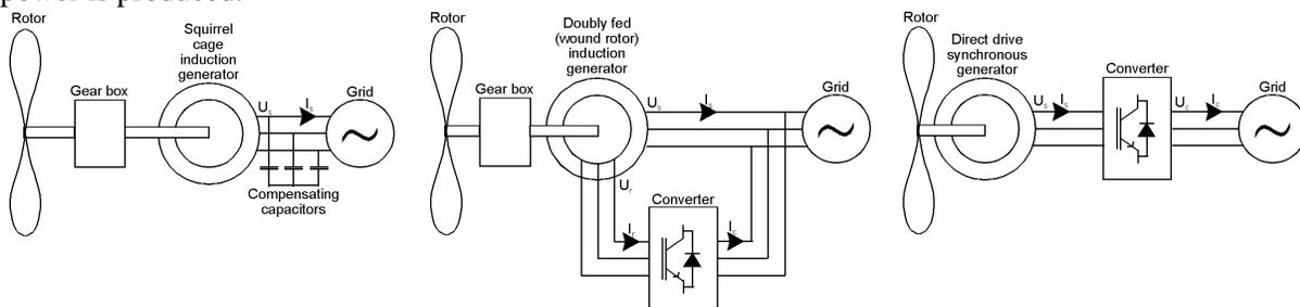
*Commonly applied generating systems in wind turbines: squirrel cage induction generator, doubly fed (wound rotor) induction generator, direct-drive synchronous generator (from the left). (From paper C6-106)*
